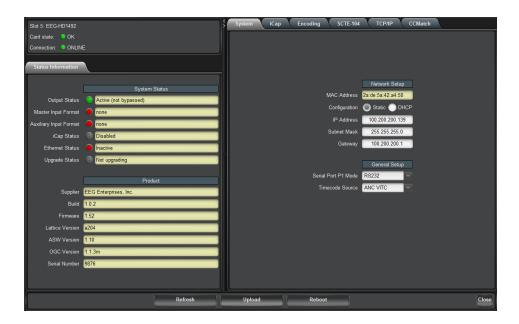
There are two main sections in the DashBoard interface: the Status information on the left side and the Setup menu on the right side. At the bottom of the interface, you will find the **Upload** button, which can be used to upgrade your HD1492's DashBoard interface firmware, and the **Reboot** button, which can be used to reboot your HD1492.
